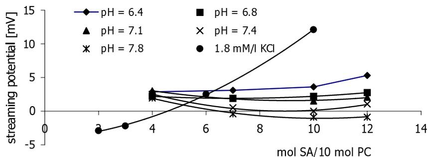
**Figure 2.** Streaming potential  $U$  for the capillary covered with membranes composed from PC/Chol (10/5 mol/mol) mixture with SA. KCl solution or phosphate buffer were used as electrolytes.
