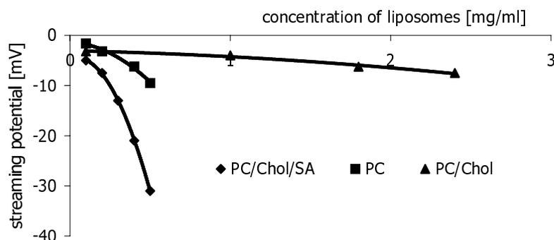
**Figure 3.** The streaming potential  $U$  for different concentrations of liposomes prepared from PC only, PC/Chol or PC/Chol/SA, all diluted in KCl. The inner surface of capillary was coated with PC/Chol/SA (2/1/1 mol././mol) lipid layer.
