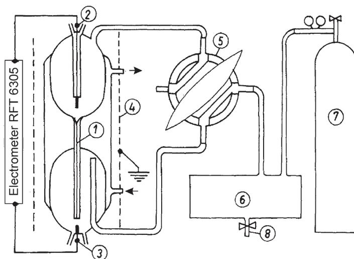
**Figure 1.** Experimental gauge and pressure-producing system for streaming potential measurements in a single capillary.
