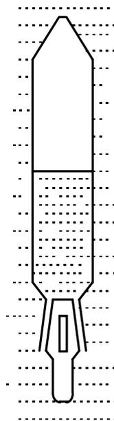
**Figure 2.** The buoy of the density meter. In the lower part there is chamber with the sample closed by a glass stopper. The stopper contains a permanent SmCo magnet.
