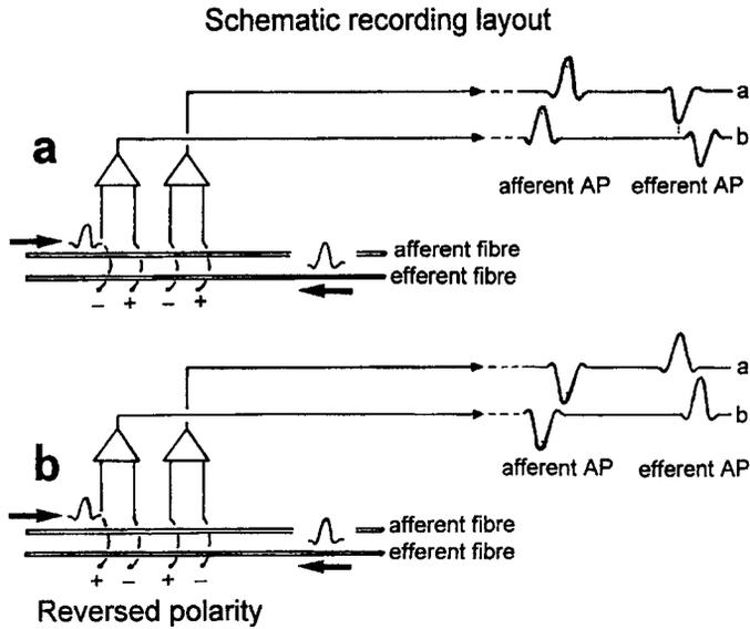
**Figure 3A:** Schematic layout for recording single-nerve fibre action potentials (APs) The reversing of the inputs to both preamplifiers does not change the ability to differentiate between afferent and efferent APs
