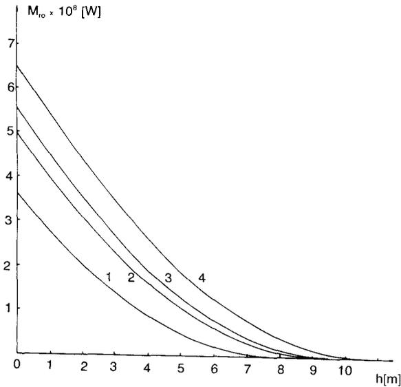
**Figure 6.** Relations  $M_{ro}(h)$  obtained for ethanol (curve 1), sucrose (curve 2), NaCl (curve 3) and  $KNO_3$  (curve 4).
