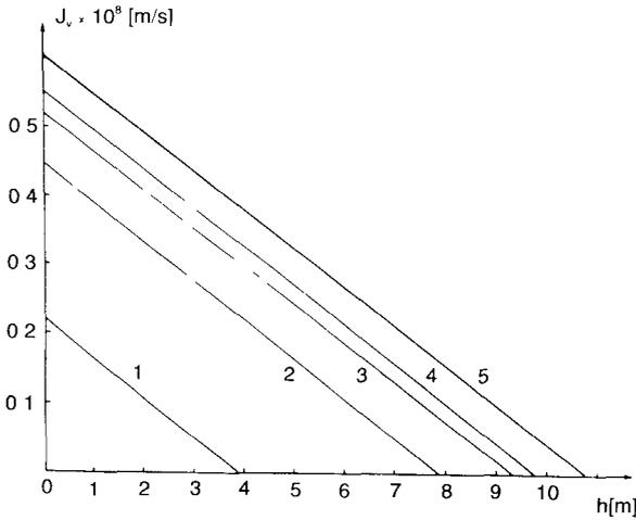
**Figure 2.** Plots of the relation  $J_v(h)$  for ethanol (curve 1), sucrose (curve 2), NaCl (curve 3),  $\text{KNO}_3$  (curve 4) and mannitol (curve 5).
