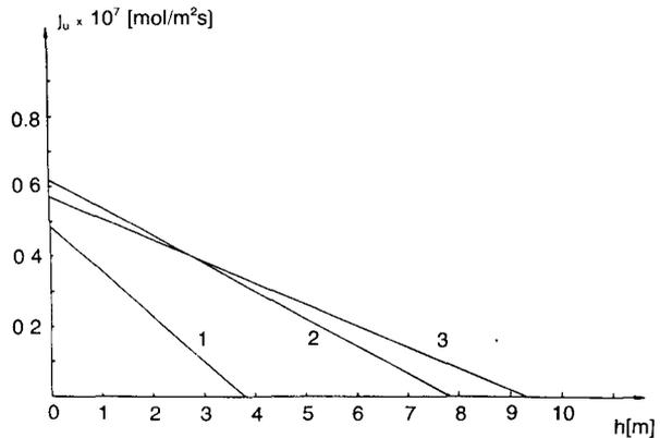
**Figure 4.** Relations  $j_u(h)$  obtained for ethanol (curve 1), sucrose (curve 2) and NaCl (curve 3).
