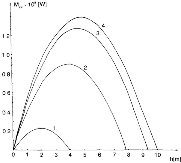
**Figure 5.** Relations  $M_{uo}(h)$  obtained for ethanol (curve 1), sucrose (curve 2), NaCl (curve 3) and  $KNO_3$  (curve 4).
