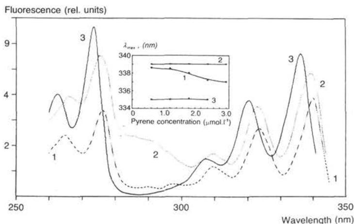
**Figure 2.** Fluorescence excitation spectra of pyrene in *P. infestans* zoospores (1,2) and in water (3). Spectra 1 and 3 were recorded at  $\lambda_{em}=397$  nm, and spectrum 2 at  $\lambda_{em}=470$  nm. Pyrene concentration:  $8 \text{ mmol.l}^{-1}$ . Insert: The dependence of excitation fluorescence maxima on pyrene concentration. The maxima positions were determined at  $\lambda_{em}=373$  nm (1,3) or at  $\lambda_{em}=470$  nm (2).
