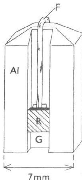
**Fig. 1.** Aluminium holder (Al) with a fibre mounted for rapid freezing. F — fibre protrusion at the top of the holder; R — a piece of rubber pressing upon the tendon; G — groove for accommodating the fibre.
