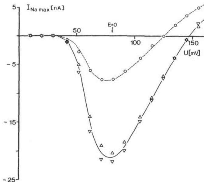
**Fig. 3.** The influence of external sodium concentration on peak sodium currents. The same experiment as in Fig. 2 but under optimum compensation of the influence of the series resistance ( $k_{\text{opt}} = 0.067$ ;  $R_s = 400 \text{ k}\Omega$ ).  $E_H = -81 \text{ mV}$ .
