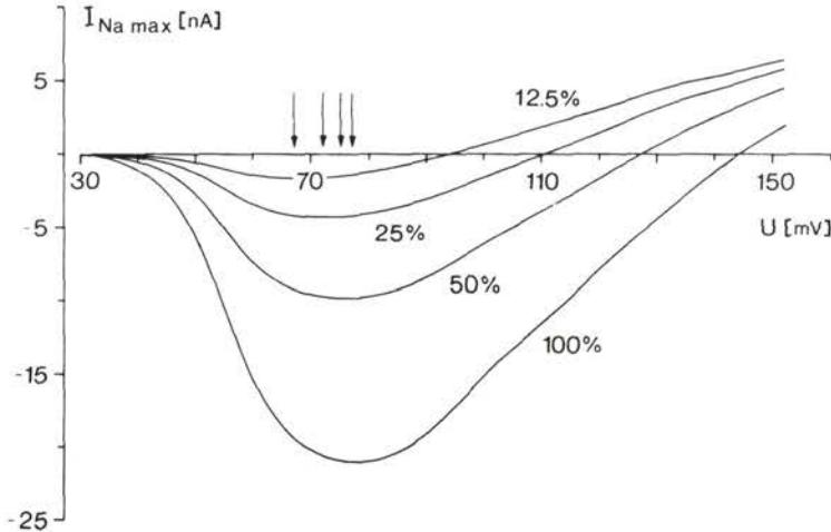
**Fig. 4.** The influence of external sodium concentration on the position of the peak sodium current-voltage curve as calculated by the independence principle. Abscissa: test pulses  $U$  in mV. Ordinate: Peak sodium currents  $I_{Na \max}$  in nA. 100%: interpolated curve for ordinary Ringer solution of Fig. 3. 50%, 25%, 12.5%: calculated curves from curve „100%“ by Eq. (1). Arrows indicate curve minima.
