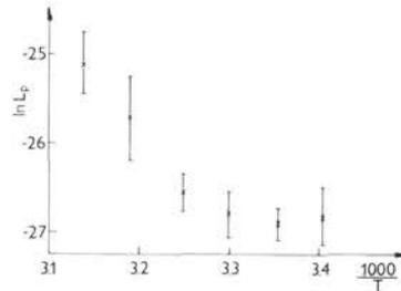
**Fig. 4.** The logarithm of the filtration coefficient plotted against  $1/T$ . The filtration coefficient is expressed in  $\text{cm}^3\text{N}^{-1}\text{s}^{-1} \times 10^{-5}$ . The values are means  $\pm$  S.D. from at least five experiments.
