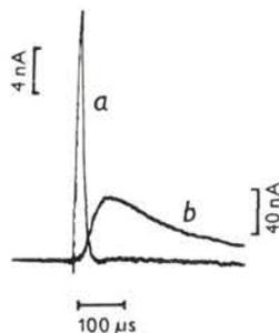
Fig. 2. Current record at a voltage jump from  $-100$  mV to  $-80$  mV (displacement 20 mV) without using the P — ( $-P/4$ ) programme (a), and current record at a voltage jump from  $-100$  mV to  $+100$  mV (displacement 200 mV) using the P — ( $-P/4$ ) programme (the current scale increased 10 times). Neuron 36.
