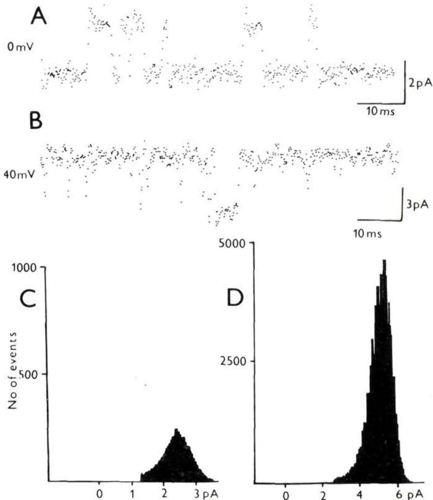
**Fig. 2.** The distribution of single channel current amplitudes. More than one hundred 512-points records such as shown in A and B were digitized with a sampling rate of 0.15 ms (i.e. 6.67 kHz). Amplitude histograms C and D obtained from data points of type A (0 mV) and B (40 mV) gave distributions with peaks of 2.4 pA and 5.6 pA respectively.
