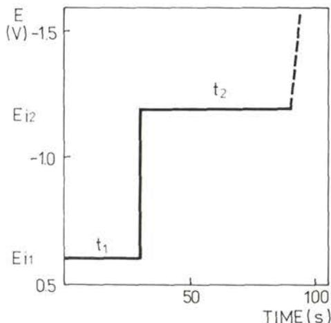
**Fig. 4.** Schematic presentation of polarization sequence of the mercury electrode with potentiostatic double step followed by single-sweep voltammetry.  $E_i$ , initial potential;  $t$ , waiting time; ---, sweep (in this paper, sweep rate was usually 0.5 V/s).
