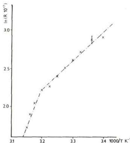
**Fig. 2.** The logarithm of the electrical resistance plotted against the reciprocal of the absolute temperature. The different slopes of the straight lines reflect a change in the activation energy at 37°C.  $R$  was expressed in  $\Omega = \text{cm}^2$ .
