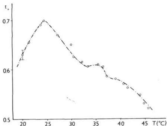
**Fig. 4.** The bulk cationic transference number plotted against the temperature. The approximate error ( $\pm 3\%$ ) is indicated.
