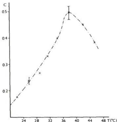
**Fig. 3.** Specific geometric capacitance plotted against the temperature. The approximate error of the measurements ( $\pm 15\%$ ) is indicated.  $C$  was expressed in  $\mu\text{F} = \text{cm}^2$ .
